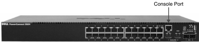
Figure 3-1. Front-Panel Console Port
